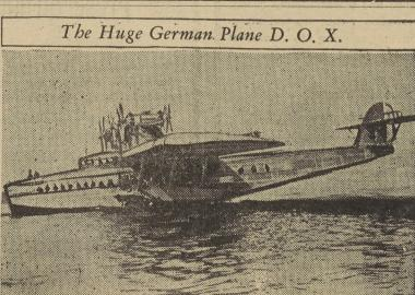
The Dorner Amphibian Plane D. O. X., Germany's pride, is equally at and members of crew. Equipped with twelve motors, it has a wing spread of one hundred and fifty feet.
