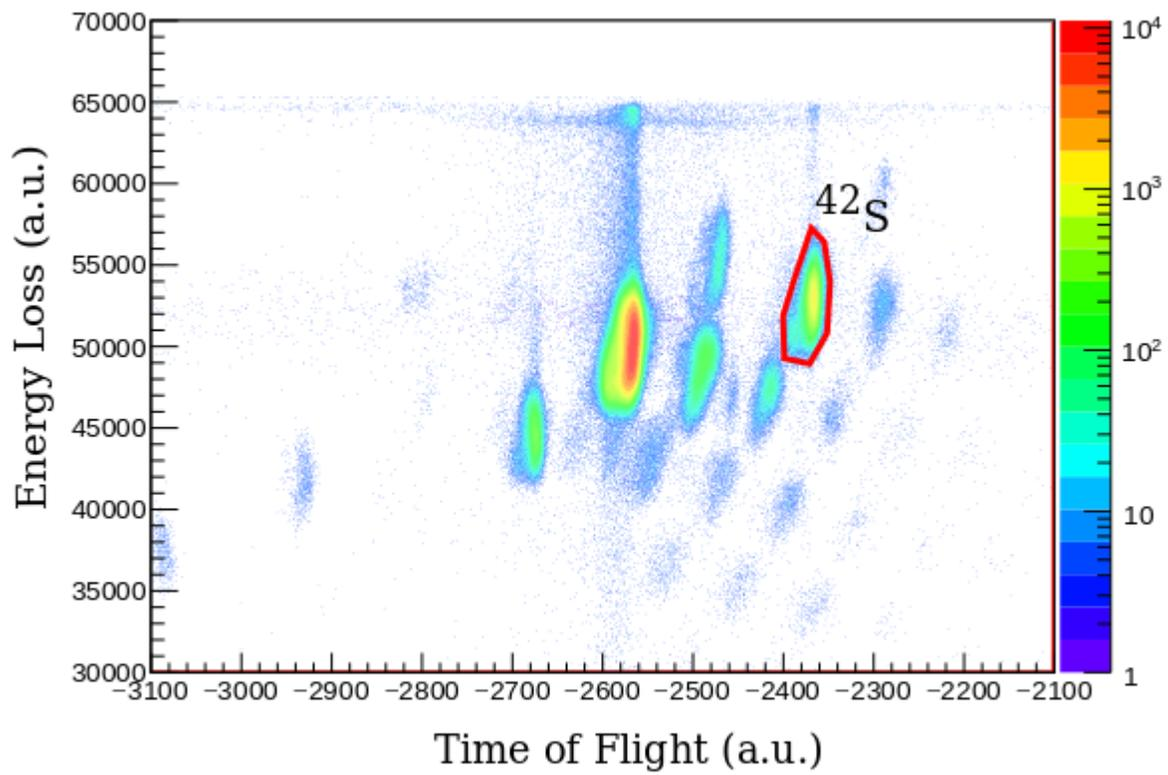
Figure 2: Outgoing particle identification spectrum generated by energy loss in the S800 ion chamber and time of flight from the S800 object scintillator to the E1 scintillator at the focal plane of the S800.
