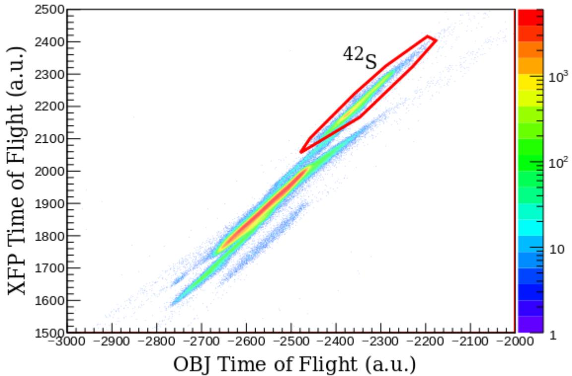
Figure 1: Incoming particle identification spectrum generated by the time of flight from the S800 object scintillator (OBJ) to the E1 scintillator in the S800 focal plane and from the A1900 extended focal plane scintillator (XFP) to the E1 scintillator.
