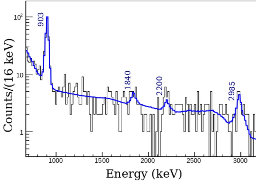
Figure 5: Doppler corrected  $\gamma$ -ray spectrum measured in coincidence with incoming and outgoing  $^{42}\text{S}$  particles. The blue curve is the fit of the GEANT4 simulations described in the text.
