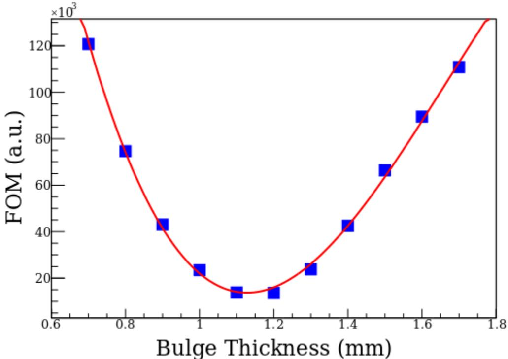
Figure 3: Simulated values for the target window bulge thickness. The red curve is a cubic polynomial fit used to minimize the function.
