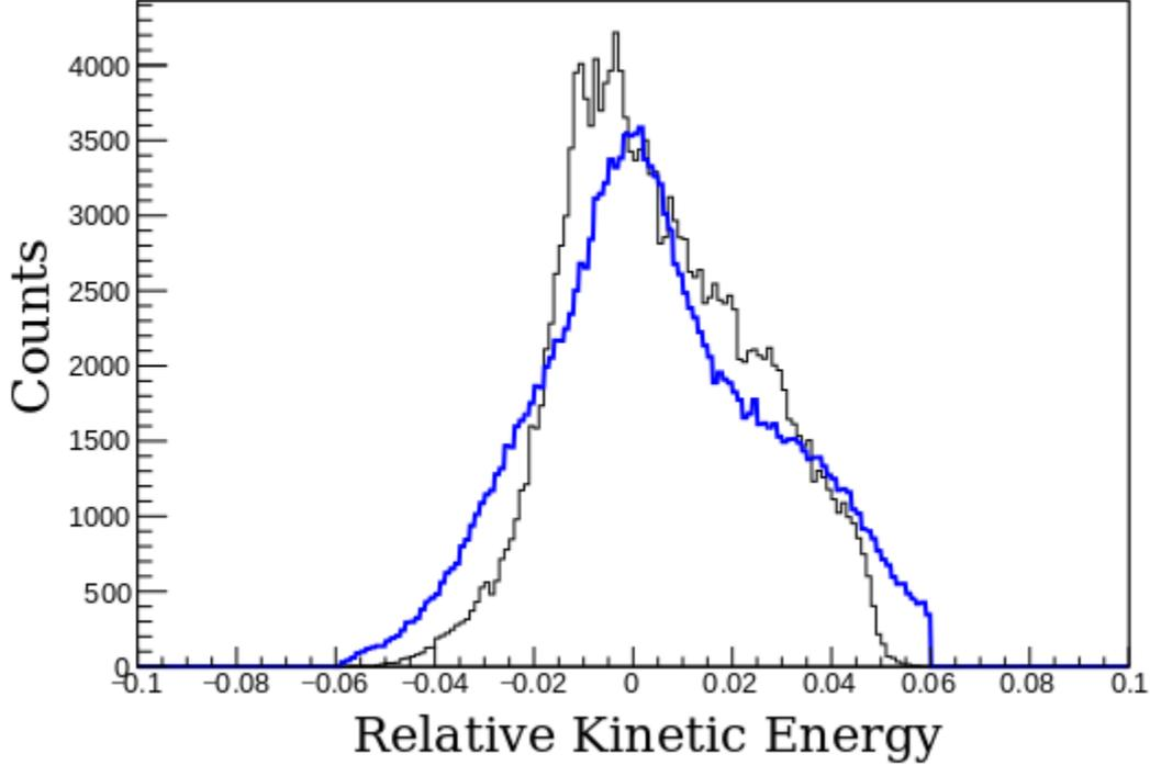
Figure 4: Relative kinetic energy spectrum of  $^{42}\text{S}$  with a simulated bulge thickness of 1.13mm.
